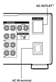
\* The configuration, shape, and number of AC outlets vary according to the model and country to which the receiver is shipped.
